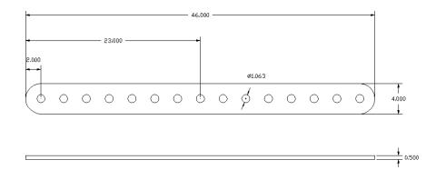
The Pull Bar (shown above) is one of a set of four required to attach the Material Spreader to the towing vehicle. The standard TRUCK MOUNTING ASSEMBLY will contain four pull bars that are 46" Long. This length should be longer than is required my almost all customers.
